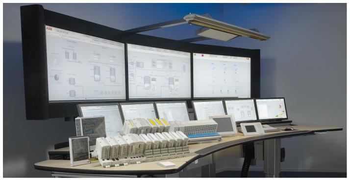
AC 800M Control and I/O provide the functionality to support the entire production facility's control requirements, from discrete and continuous to batch and advanced control and safety applications.
