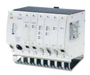
The AC 800F controller has a modular structure. The CPU is designed as a backplane to which various modules - power supply units, Ethernet and fieldbus modules - can be attached in line with the application. On the fieldbus side, modules for PROFIBUS-DPV1, FOUNDATION Fieldbus HSE, MODBUS (master / slave, RTU or ASCII), IEC 60870-5-101, IEC 60870-5-104 and CAN for Freelance Rack I/O are available.
